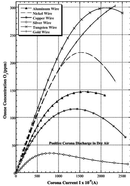
Fig. 6. The ozone concentration generated by the positive corona discharge in dry air as a function of the corona current for different materials of the wire.
