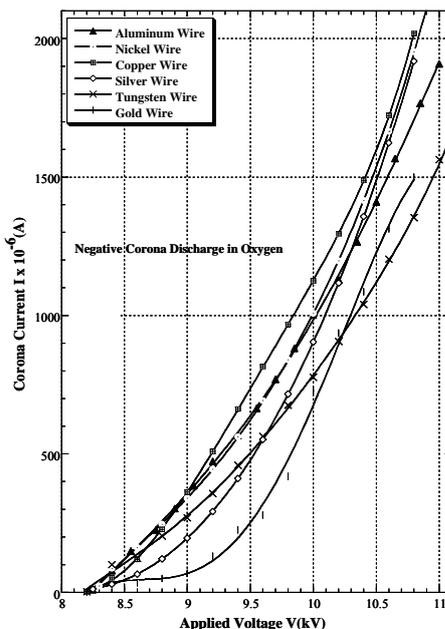
Fig. 5. Current-voltage characteristics of the negative corona discharge in oxygen for different materials of the wire.
