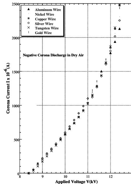
Fig. 3. Current-voltage characteristics of the negative corona discharge in dry air for different materials of the wire.
