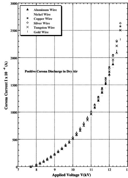
Fig. 2. Current-voltage characteristics of the positive corona discharge in dry air for different materials of the wire.
