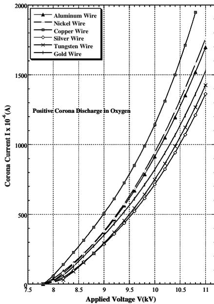
Fig. 4. Current-voltage characteristics of the positive corona discharge in oxygen for different materials of the wire.
