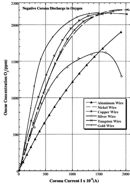
Fig. 9. The ozone concentration generated by the negative corona discharge in oxygen as a function of the corona current for different materials of the wire.
