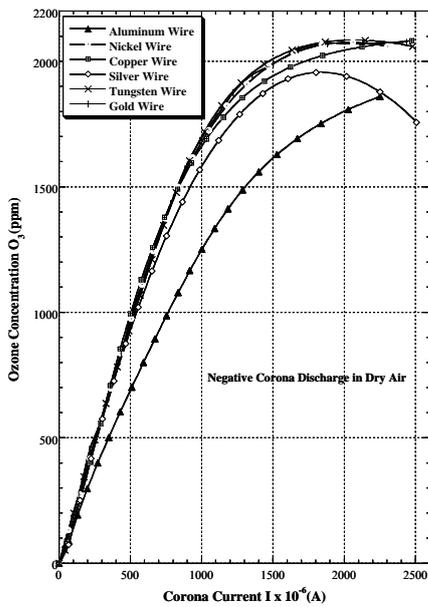
Fig. 7. The ozone concentration generated by the negative corona discharge in dry air as a function of the corona current for different materials of the wire.
