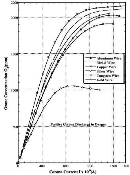
Fig. 8. The ozone concentration generated by the positive corona discharge in oxygen as a function of the corona current for different materials of the wire.
