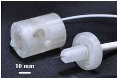
Fig. 3. 3D-printed single-IWD with variable gap distance.
